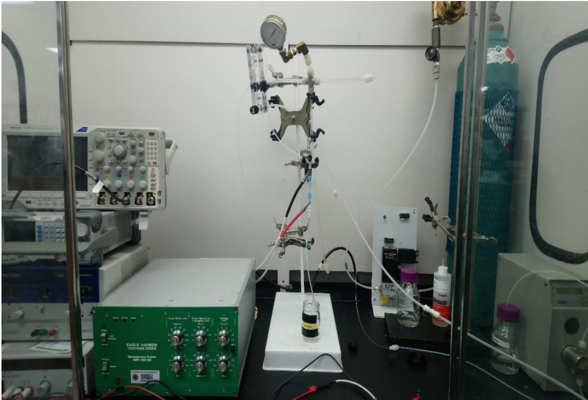
Figure 2. The plasma reactor used in this study
